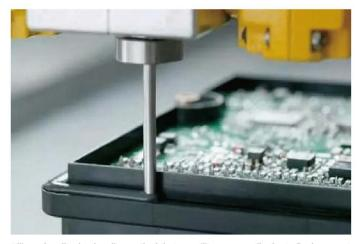
Silicone bonding is a bonding method that uses silicone as an adhesive to firmly connect two surfaces together. It has excellent adhesive performance and high temperature resistance, can cure at room temperature, and is suitable for various material surfaces.
