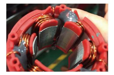
Motor assembly, magnetic tile fixation, and inverter wire fixation
